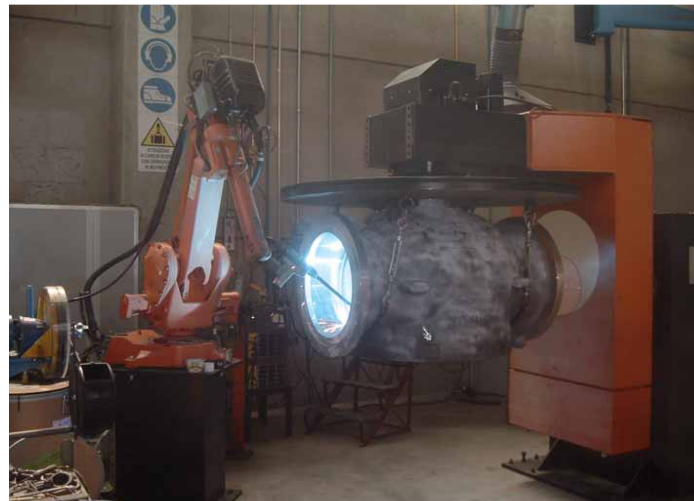
Corpo 24" 150 - Riporto integrale Inconel 625 - Procedimento a Filo GMAW Body Top Entry 24" 150 - Inconel 625 Full Overlay - GMAW Process.
