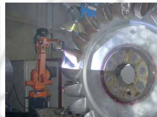
Girante Pelton - Overlay Pale Inox 13/4 - Procedimento Filo GMAW Pelton Runner - Inside Bucket Inox 13/4 Overlay - GMAW Process
