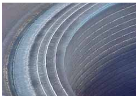
Overlay Inconel 625 Procedimento Filo GMAW Inconel 625 Overlay - GMAW Process
