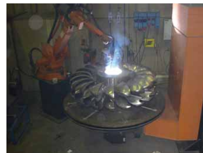
Girante Pelton - Overlay diametro Interno Inox 13/4 - Procedimento Filo GMAW Pelton Runner - Internal Diameter Inox 13/4 Overlay - GMAW Process
