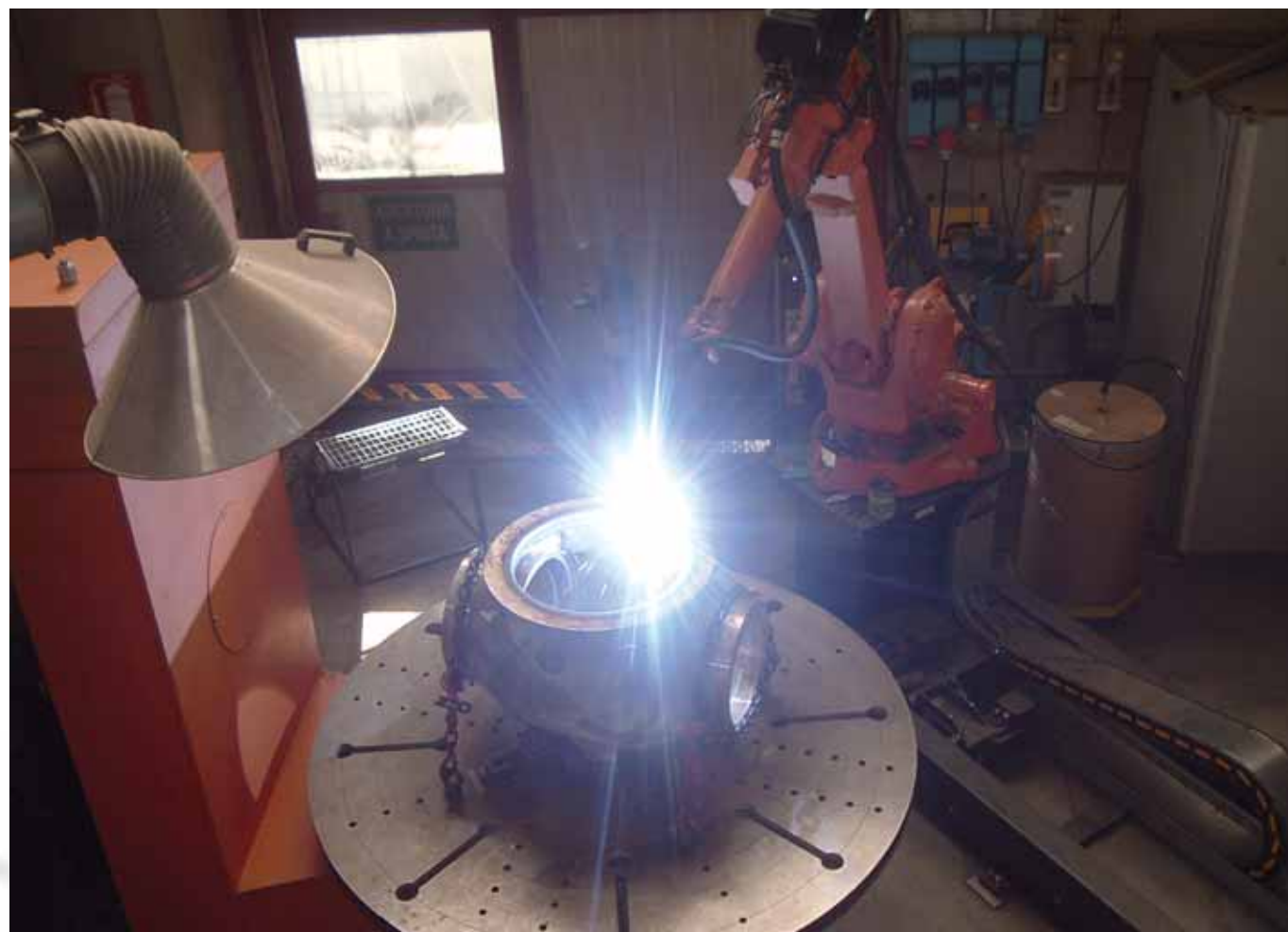
Corpo Valvola Top Entry 12" - Overlay totale Inconel 625 - Procedimento Filo GMAW Body Top Entry 12" - Inconel 625 Full Overlay - GMAW Process
