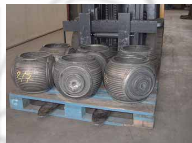
Sfere 8" - Overlay Inconel 625 - Procedimento Filo GMAW Ball 8" - Inconel 625 Overlay - GMAW Process
