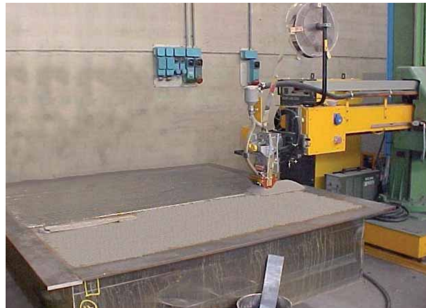
Placcatura Anticorrosione su Piani e Piastre Strip Plating against corrosion and wear on Plates
