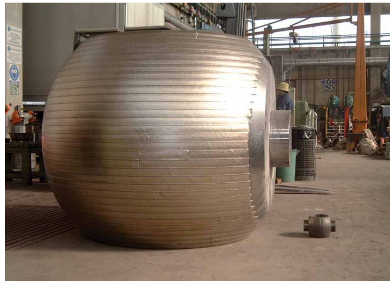
Sfera 52" - Overlay Inox 309/316 - Procedimento Arco Sommerso SAW Sfera 6" - Overlay Inconel 625 - Procedimento a Filo GMAW Ball 52" - Stainless Steel 309/316 Overlay - Submerged Arc Process Ball 6" - Inconel 625 Overlay - GMAW Process
