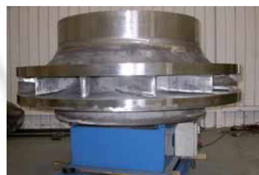
Girante Francis - Finita dopo ripristino. Francis Runner - Finished after Inox 13/4 Overlay
