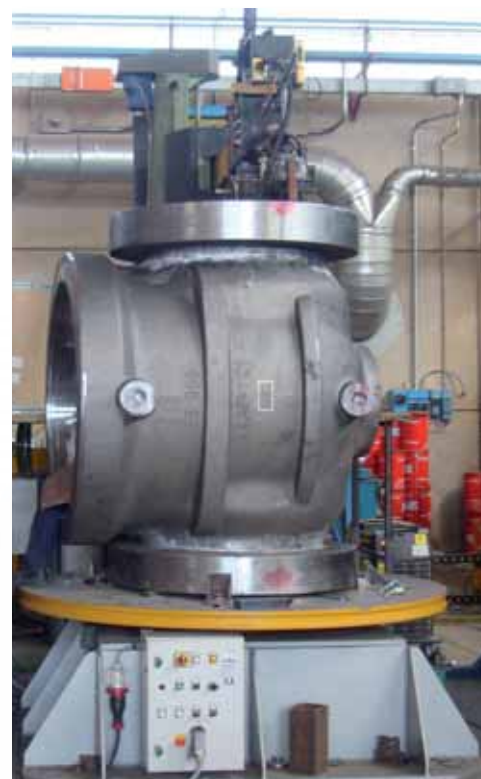
Corpo Top Entry 28" 900 Overlay Inconel 625 Procedimento GMAW Body Top Entry 28" 900 - Inconel 625 Overlay - GMAW Process
