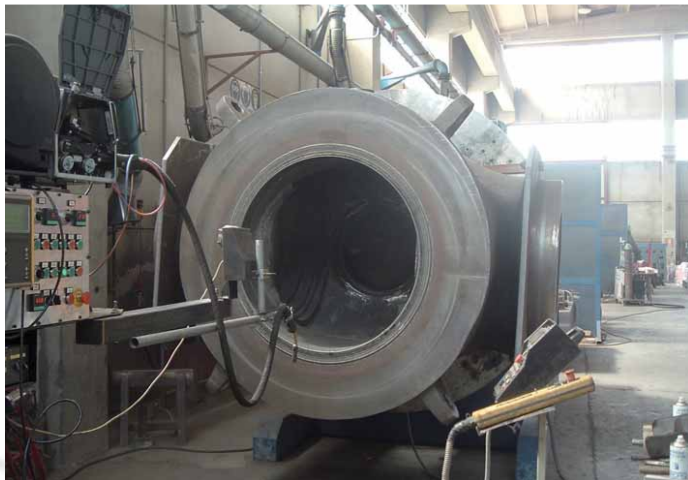
Corpo Valvola Top Entry 38" 900 - Overlay totale Inconel 625 - Procedimento Filo GMAW Body Top Entry 38" 900 - Inconel 625 Full Overlay - GMAW Process
