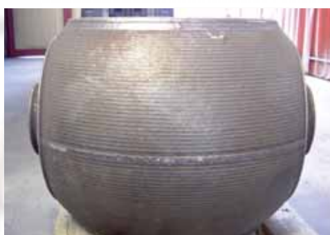
Sfera 28" - Overlay totale Inox 309/316 - Procedimento Filo Ball 28" - Stainless Steel 309/316 Overlay - GMAW Process
