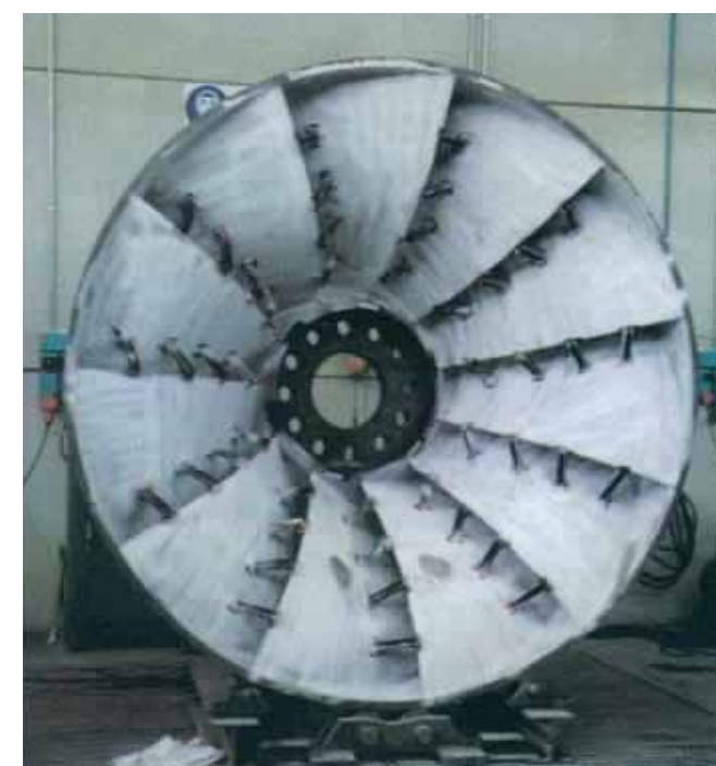
Girante Francis in lavorazione Francis Runner in progress
