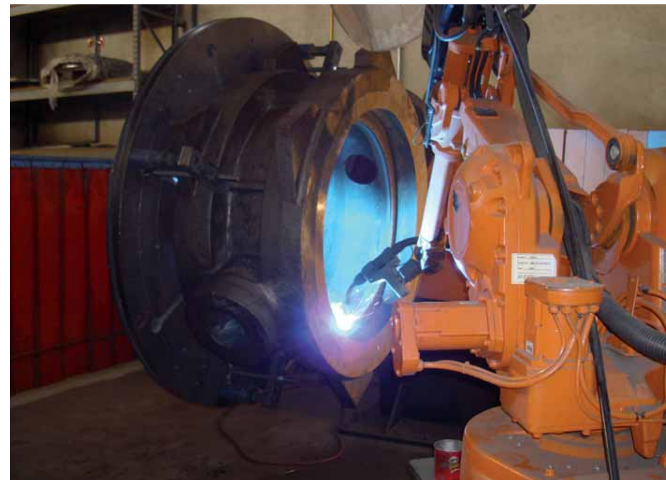
Valvola Butterfly 42" - Overlay Inox 316 Seggio Ellittico - Procedimento Filo GMAW Butterfly Valve 42" - Stainless Steel 316 Overlay Elliptical Ring Joint - GMAW Process
